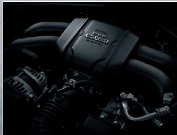
Horizontally-opposed Boxer engine
